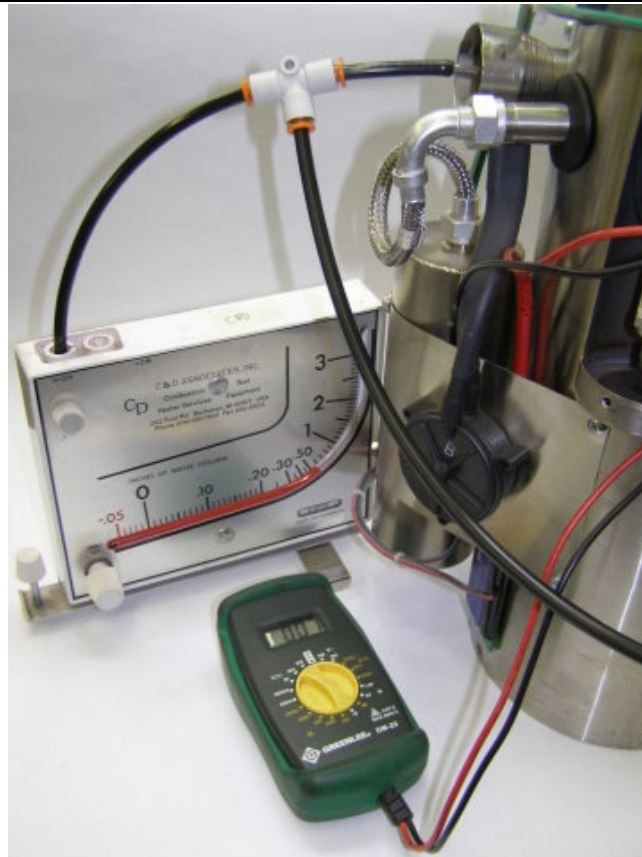
FIGURE 27A: COMBUSTION AIR SWITCH TESTING
